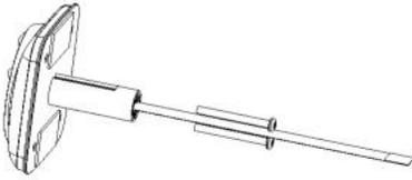
Choose appropriate screw length based on door thickness. Then twist it into the screw hole.
